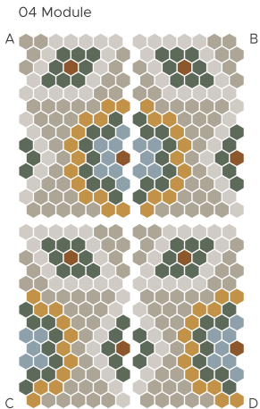
HEXA MINI-50 Module : A, B, C, D - 175x291mm / 0.51 sq. ft. Gap : 2mm | Chip Size : 22x25mm
